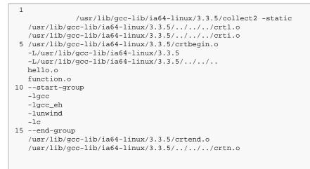
The first thing you notice is that a program called collect2 is being called. This is a simple wrapper around ld that is used internally by gcc.
